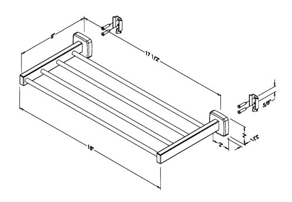
THE EUROPA II SERIES BATH ACCESSORIES ARE FABRICATED OF TYPE 304 STAINLESS STEEL AND ARE AVAILABLE IN THE FOLLOWING FINISHES:
