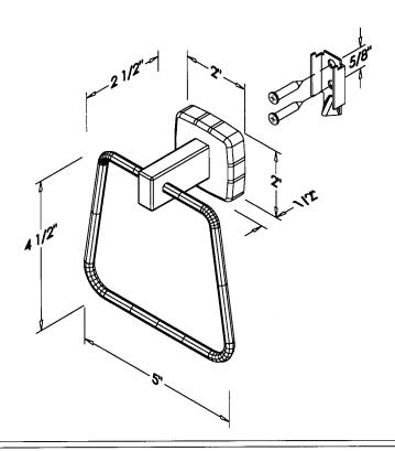
THE EUROPA II SERIES BATH ACCESSORIES ARE FABRICATED OF TYPE 304 STAINLESS STEEL AND ARE AVAILABLE IN THE FOLLOWING FINISHES:
