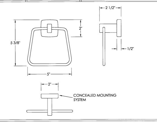
THE EUROPA II SERIES BATH ACCESSORIES ARE FABRICATED OF TYPE 304 STAINLESS STEEL AND ARE AVAILABLE IN THE FOLLOWING FINISHES:
