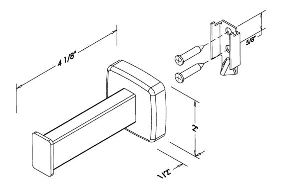
THE EUROPA II SERIES BATH ACCESSORIES ARE FABRICATED OF TYPE 304 STAINLESS STEEL AND ARE AVAILABLE IN THE FOLLOWING FINISHES:
