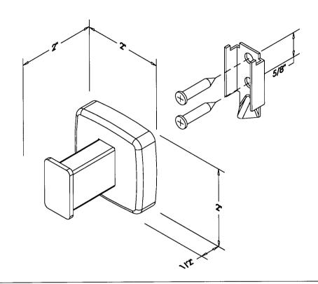
THE EUROPA II SERIES BATH ACCESSORIES ARE FABRICATED OF TYPE 304 STAINLESS STEEL AND ARE AVAILABLE IN THE FOLLOWING FINISHES:
