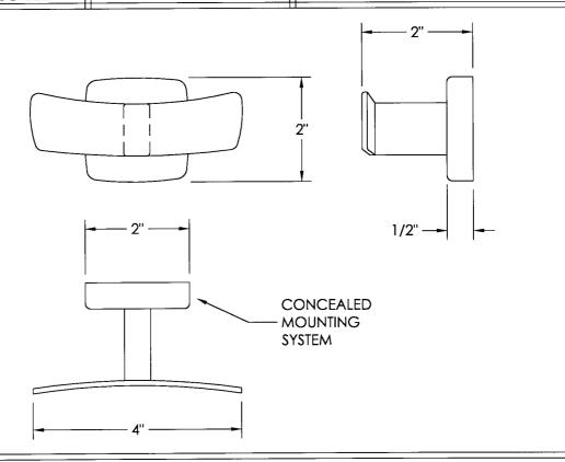
THE EUROPA II SERIES BATH ACCESSORIES ARE FABRICATED OF TYPE 304 STAINLESS STEEL AND ARE AVAILABLE IN THE FOLLOWING FINISHES:
