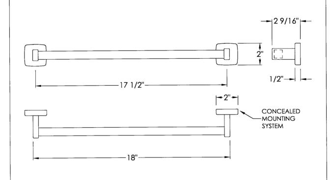
THE EUROPA II SERIES BATH ACCESSORIES ARE FABRICATED OF TYPE 304 STAINLESS STEEL AND ARE AVAILABLE IN THE FOLLOWING FINISHES:
