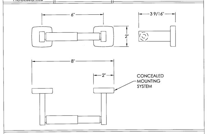
THE EUROPA II SERIES BATH ACCESSORIES ARE FABRICATED OF TYPE 304 STAINLESS STEEL AND ARE AVAILABLE IN THE FOLLOWING FINISHES:
