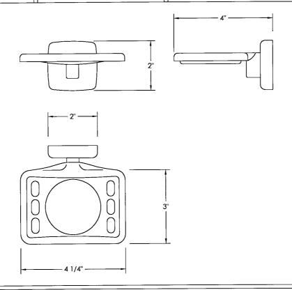
THE EUROPA II SERIES BATH ACCESSORIES ARE FABRICATED OF TYPE 304 STAINLESS STEEL AND ARE AVAILABLE IN THE FOLLOWING FINISHES:
