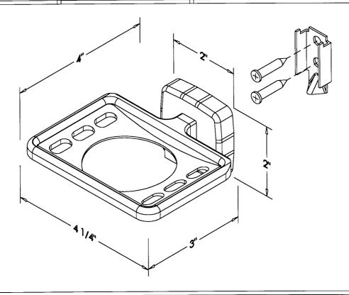
THE EUROPA II SERIES BATH ACCESSORIES ARE FABRICATED OF TYPE 304 STAINLESS STEEL AND ARE AVAILABLE IN THE FOLLOWING FINISHES:
