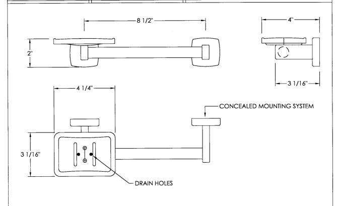
THE EUROPA II SERIES BATH ACCESSORIES ARE FABRICATED OF TYPE 304 STAINLESS STEEL AND ARE AVAILABLE IN THE FOLLOWING FINISHES:
